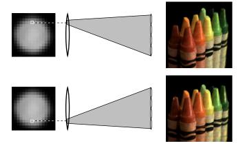
**Figure 4:** Two sub-aperture photographs obtained from a light field by extracting the shown pixel under each microlens (depicted on left). Note that the images are not the same, but exhibit vertical parallax.
