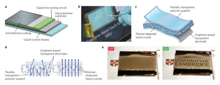
Figure 4 | Graphene touch screen and smart window. a, Schematic of a capacitive touch screen. b, Resistive graphene-based touch screen. c, Schematic of a PDLC smart window using a GTCF. d, With no voltage, the liquid-crystal molecules are not aligned, making the window opaque. e, Graphene/nanotube-based smart window in either an off (left) or on (right) state. Image in b reproduced with permission from ref. 39, © 2010 NPG.
