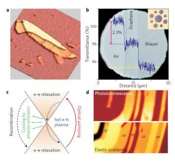
Figure 1 | The optical properties of graphene. a, Elastic light scattering (Rayleigh) image of a graphite flake with varying number of graphene layers<sup>9</sup>. b, Transmittance for an increasing number of layers. Inset, sample design for the experiment of ref. 11, showing a thick metal support structure with several apertures, on top of which grahene flakes are placed.
